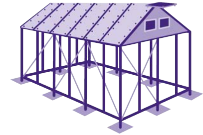
7. Add pipes and cross wires
